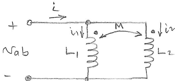
$$v_{ab} = L_1 \frac{di_1}{dt} + M \frac{di_2}{dt} \quad \text{for coil 1.} \quad (1)$$
