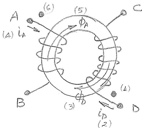
The following 6 steps are applied to determine the dot markings:
