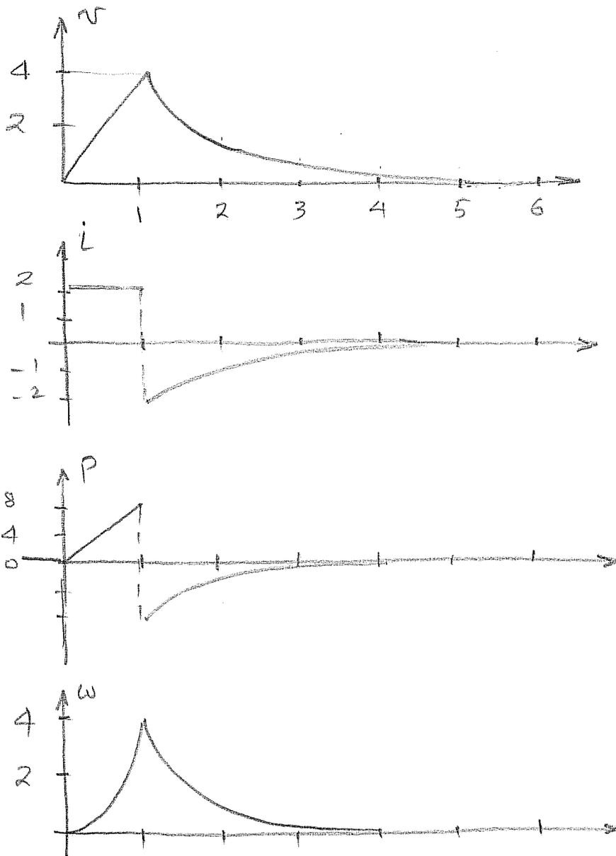
When  $p > 0$  energy is being stored in the capacitor ( $v$  increases and  $w$  increases). When  $p < 0$  energy is being delivered by the capacitor ( $w$  is decreasing). The area under the  $p$ -curve is the energy delivered to the capacitor when  $p > 0$  ( $t < 1$  s), and the area under the  $p$ -curve when  $t > 1$  s is the energy delivered by the capacitor.
