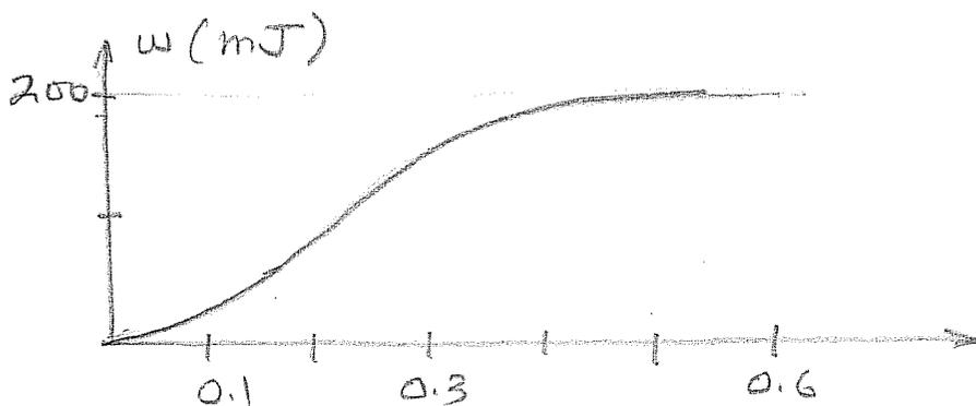
The energy in the inductor is not dissipated (no resistance). The energy approaches 200 mJ as  $t \rightarrow \infty$  because the current approaches 2A as  $t \rightarrow \infty$ !
