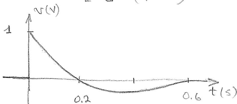
Note the voltage has a zero value at the maximum of the current. At this instant there is a change of polarity.
