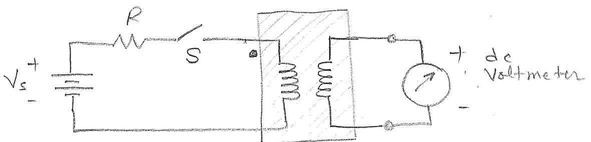
A dot is placed on the terminal of coil 1 connected to the positive pole of the battery. When switch  $S$  is closed, the voltmeter (momentary) deflection is observed. If the deflection is upscale, the terminal connected to the positive terminal of the voltmeter receives the dot mark. If the deflection is downscale, the terminal connected to the negative terminal of the voltmeter receives the dot mark.
