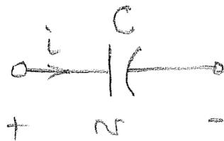
The current is proportional to the rate of change of voltage with respect to time:
