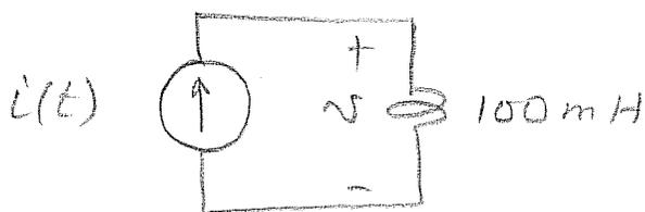
a) Draw  $i(t)$  and determine  $t_{\max}$  when  $i(t)$  is maximum.
