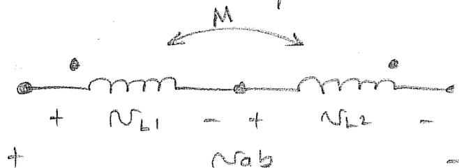
$$v_{L1} = L_1 \frac{di}{dt} - M \frac{di}{dt} \quad \text{and} \quad v_{L2} = L_2 \frac{di}{dt} - M \frac{di}{dt}$$
