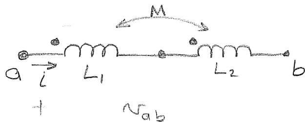
The voltage  $v_{ab} = v_{L1} + v_{L2}$
