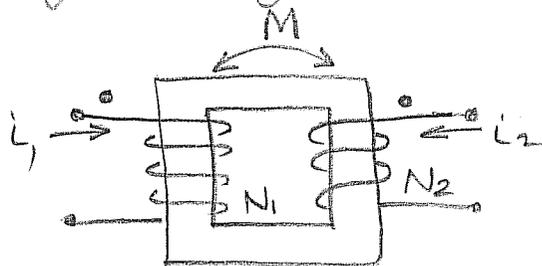
Let  $L_1$  and  $L_2$  be the self inductances of coils 1 and 2. It can be shown that the mutual inductance  $M$  of the two coils is given by:
